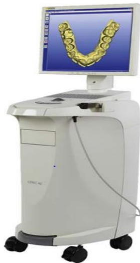
FIG. 11.6 Chair-side computer-aided design/computer-aided manufacturing system for all-ceramic restorations fabrication. (Courtesy Sirona Dental Systems, LLC, Charlotte, NC.)
