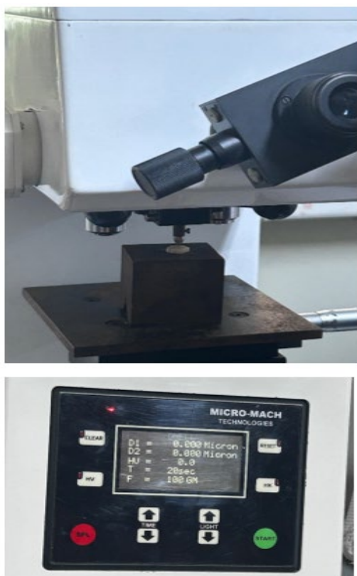
Figure 5: Stabilization of composite resin blocks in Vickers Microhardness Tester and recording of Vickers hardness number under digital microscopy
